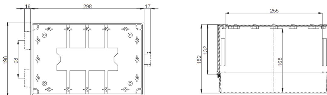
The housing is mounted using four brackets (mounting points in the corners of the enclosure).
