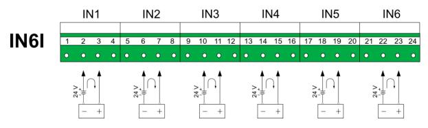
Fig. 6.4 IN6I module output transducer wiring diagram.
