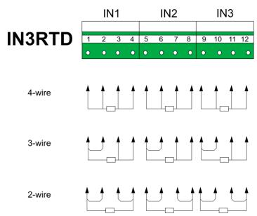
Fig. 6.6 RTD sensor wiring to IN3RTD module diagram.
