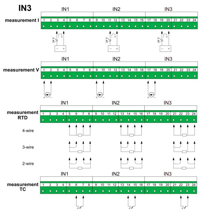
Fig. 6.9 Wiring diagram for IN3 module.
