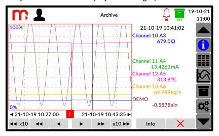
Fig. 11.13 An example view of the 'View Archive' window – packet with error value.
