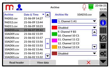
Fig. 11.10 An example view of the 'View Archive' window - selecting the data to be displayed.
