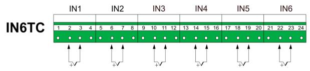
Fig. 6.7 Thermocouple wiring to IN6TC module diagram.
