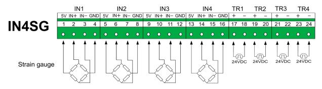
Fig. 6.12 Wiring diagram for IN4SG module.
