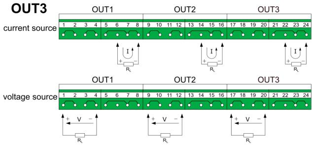
Fig. 6.18 Wiring diagram for OUT3 module.
