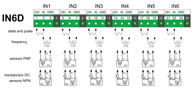
Fig. 6.23 Wiring diagram for IN6D module.
