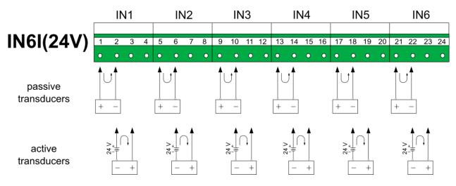
Fig. 6.3 IN6I(24V) module output transducer wiring diagram.
