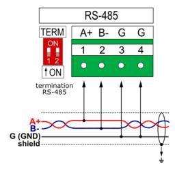
Fig. 6.22 Wiring diagram for RS-485.
