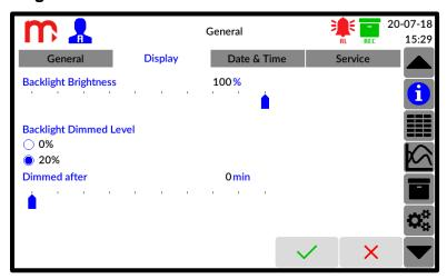
Fig. 12.1 An example view of the 'General' settings window - 'Display' tab.
