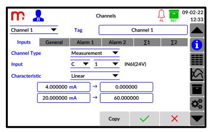
Fig. 12.4 An example view of the 'Channel' settings window (math channel).
