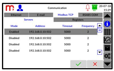
Fig. 12.3 An example view of the 'Communication' settings window.
