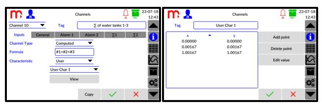
Fig. 14.2 An example view of the 'Channel' settings window (edition of user characteristics).
