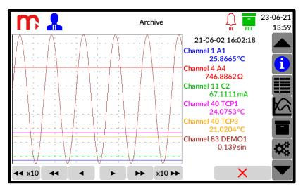
Fig. 11.11 An example view of the 'View Archive' window - data displaying.
