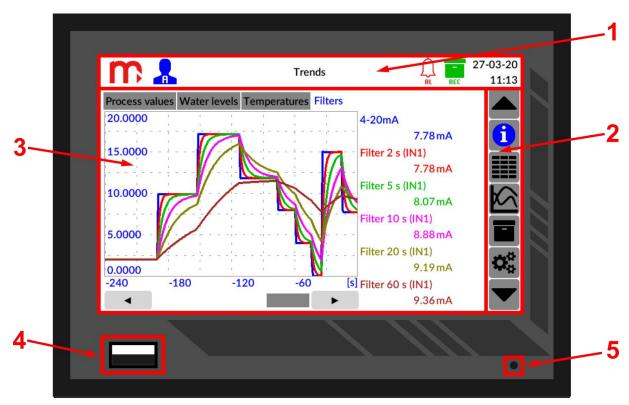
Fig. 7.1 Front panel of the device.
