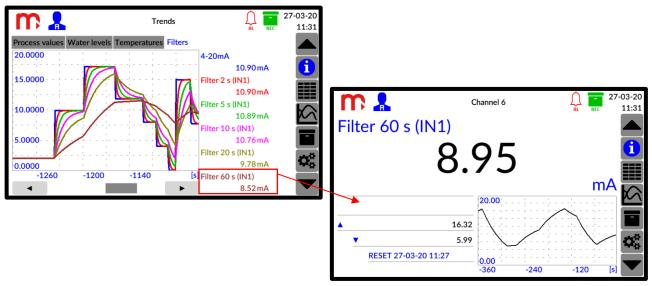
Fig. 11.5 Toggling from the 'Trends' window to a Single Result window.
