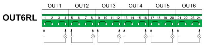
Fig. 6.17 Wiring diagram of receivers to relay outputs of OUT6RL module.
