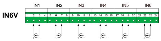
Fig. 6.8 Wiring diagram of transducers to IN6V module.
