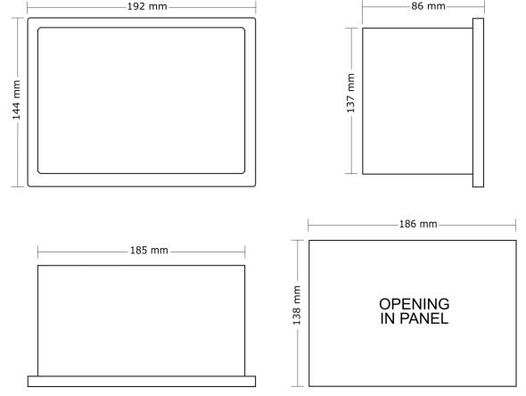
Fig. 5.1 Housing dimensions of DL7 device and cut-out dimensions in an assembly panel.
