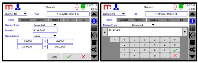
Fig. 14.1 Settings of math channels - entering the formula of the math channel.
