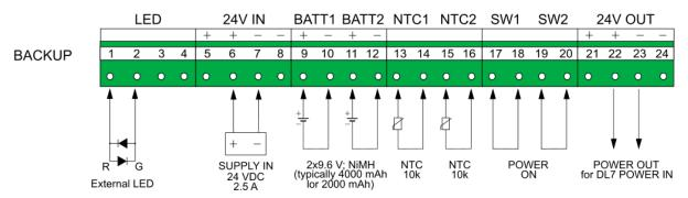
Fig. 6.21 Wiring diagram for PSBATT module.
