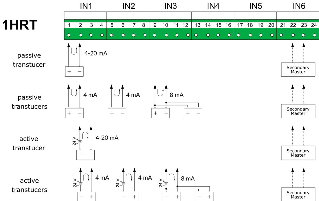
Fig. 6.16 1HRT module output transducer wiring diagram.
