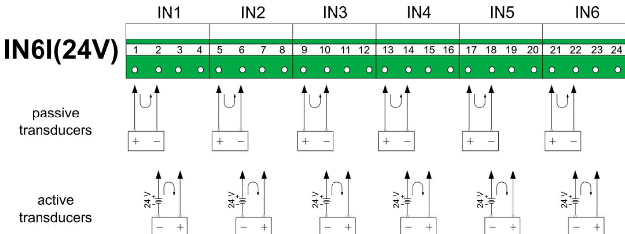
Fig. 6.3 IN6I(24V) module output transducer wiring diagram.
