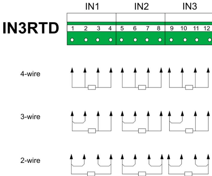
*Fig. 6.6 RTD sensor wiring to IN3RTD module diagram.*
