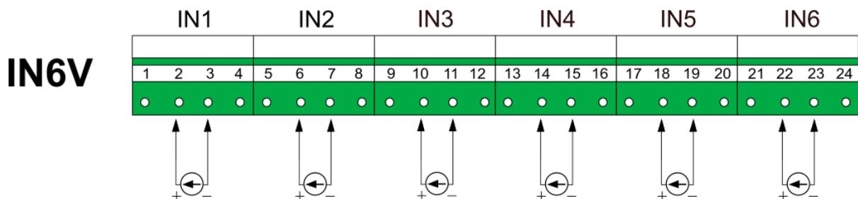
Fig. 6.8 Wiring diagram of transducers to IN6V module.
