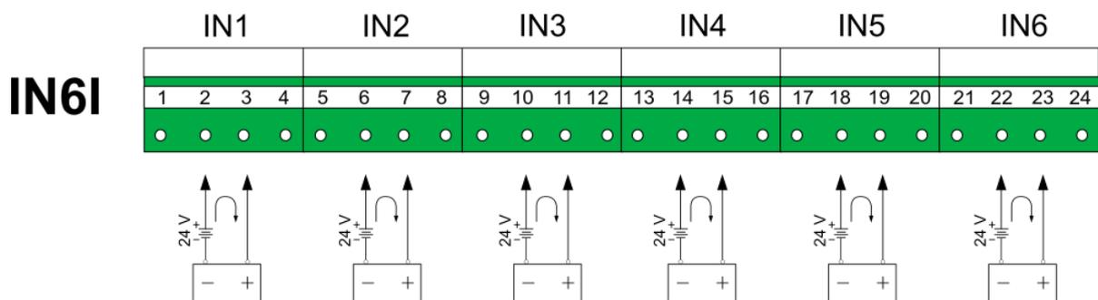
Fig. 6.4 IN6I module output transducer wiring diagram.
