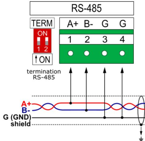
Fig. 6.22 Wiring diagram for RS-485.
