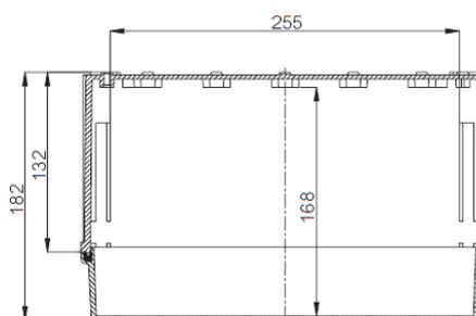
The housing is mounted using four brackets (mounting points in the corners of the enclosure).
