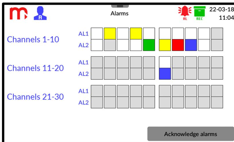
Fig. 11.9 An example view of the 'Alarms' window.
