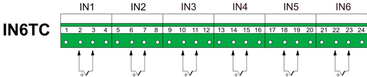
*Fig. 6.7 Thermocouple wiring to IN6TC module diagram.*
