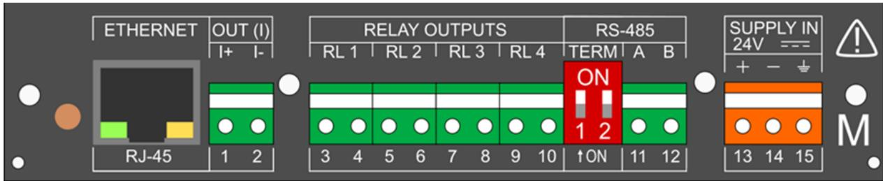
Fig.6.21 Model view of the rear plate of DL2 (module M).
