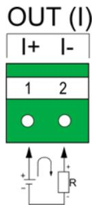
Fig. 6.22 Wiring diagram for the analog output.
