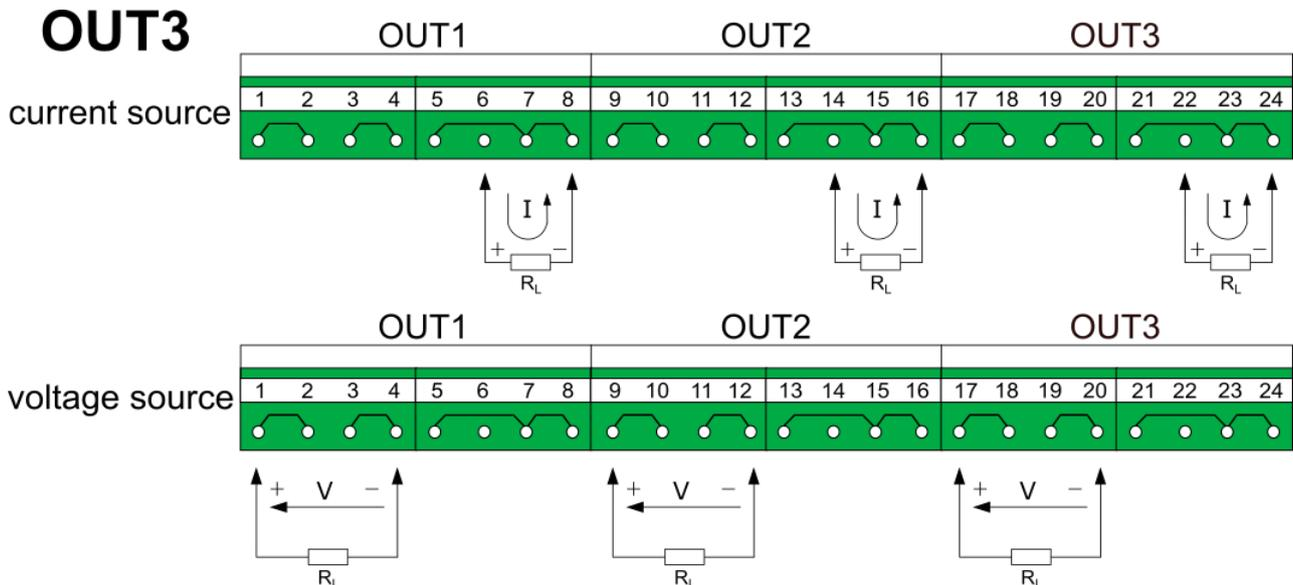
Fig. 6.17 Wiring diagram for OUT3 module.
