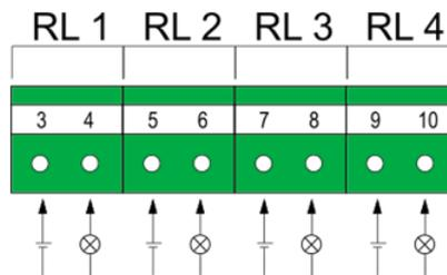
Fig. 6.23 Wiring diagram for the relay outputs.
