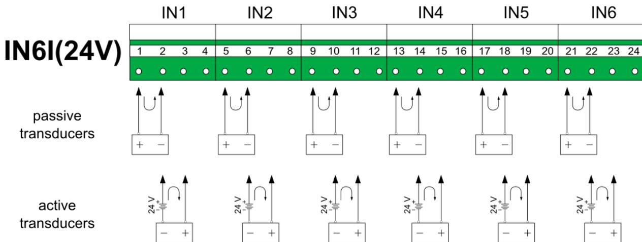
Fig. 6.3 IN6I(24V) module output transducer wiring diagram.
