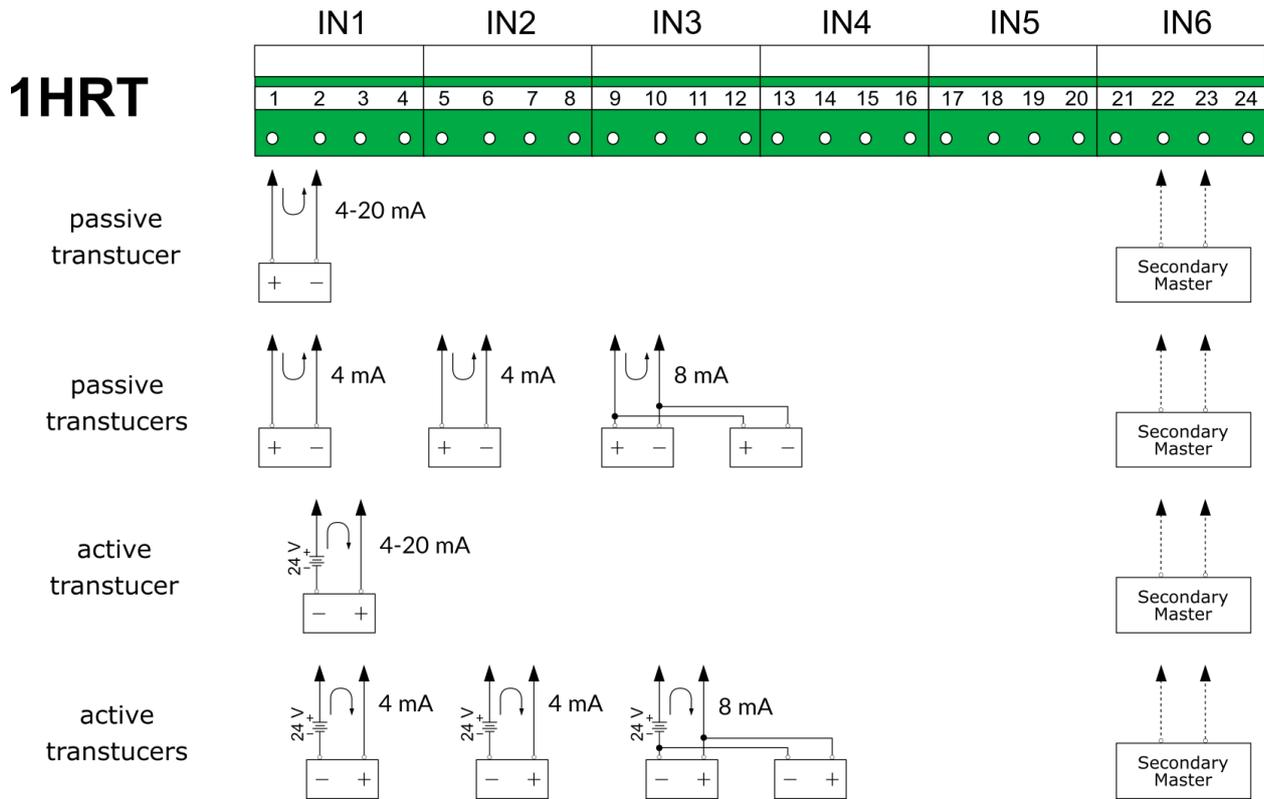
Fig. 6.15 1HRT module output transducer wiring diagram.
