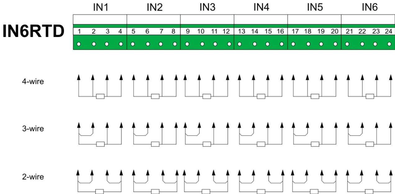
*Fig. 6.5 RTD sensor wiring to IN6RTD module diagram.*
