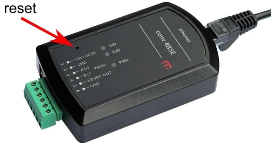
*Figure 3.5 RESET button location*
