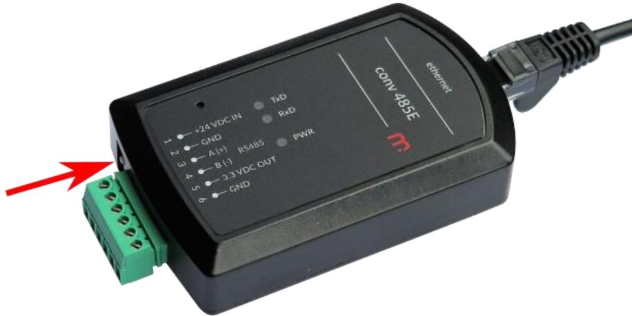
Figure 2.1 Termination switch location
