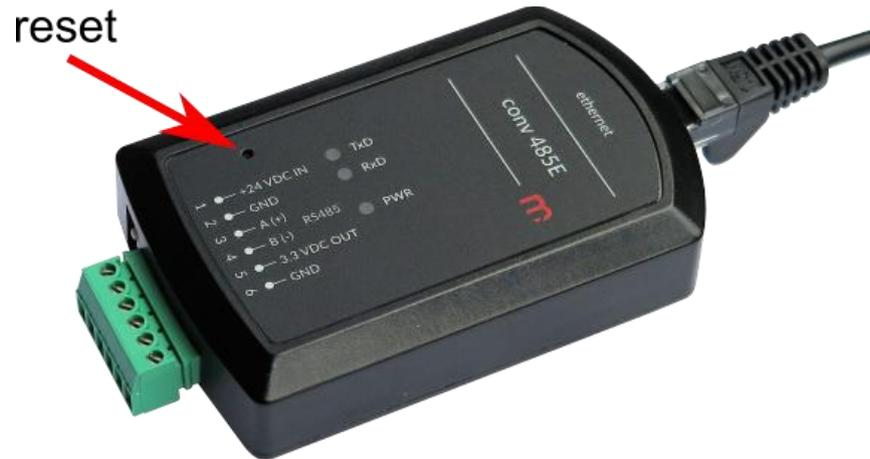
*Figure 3.5 RESET button location*
