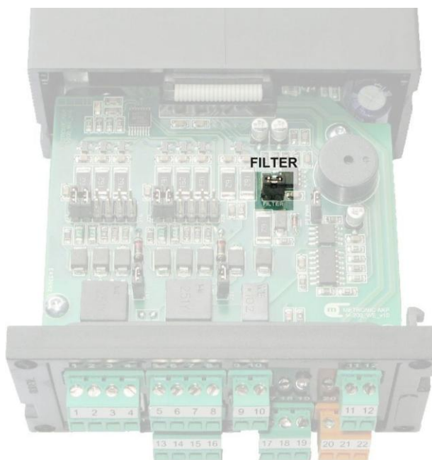
Fig. 2.10 Filter activating/deactivating jumper
