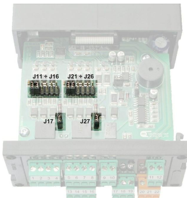
Fig. 2.9 Jumpers for analogue input configuration
