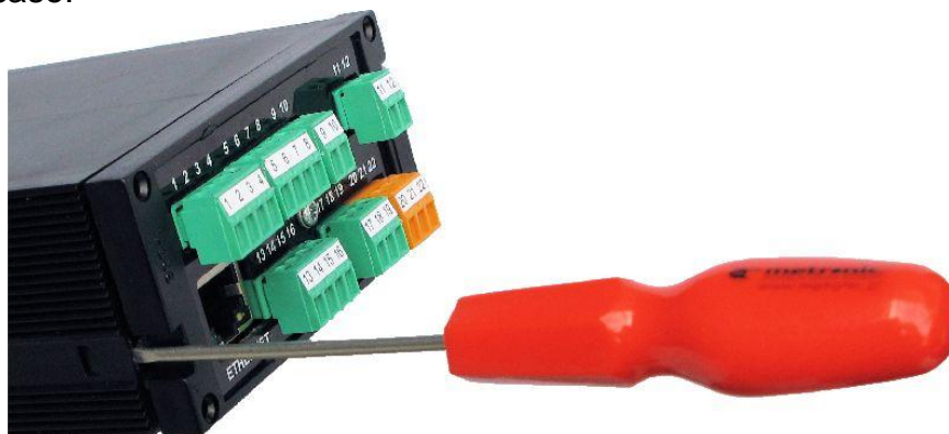
Fig. 2.8 Case disassembly
