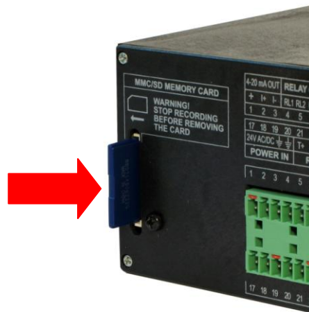
FP-3010. MMC/SD card socket; Socket in FP-3010 is situated similarly.
